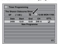
5 Press [I/O ON/STANDBY] to go to the timer-standby mode.
