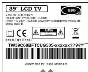
EXAMPLE OF LABEL ON REAR OF TV
