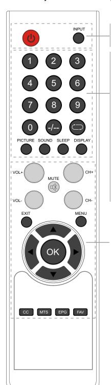
**OPENICATION** POWER(red button): Turn the TV on/standby. INPUT: Press to display the input source menu.
