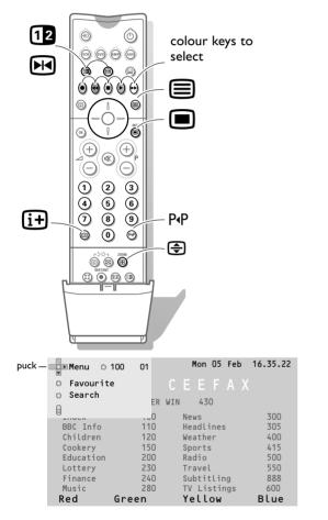
The main index page appears on the screen together with an information line at the top, an option line at the bottom and a puck in the top left corner of the screen.
