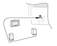
Connect two rear loudspeakers with built in amplifiers or an audio amplifier with rear loudspeakers. Connect the audio cables to the rear loudspeakers and to the Dolby surround output **S**
