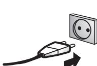
Insert the mains plug into a wall socket (220-240 V / 50 Hz).
