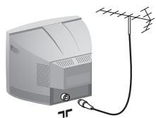
Insert the aerial plug into the socket at the rear of the set.
