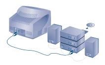
To connect to a hi-fi system, use an audio connection cable and connect the "L" and "R" outputs on the TV set to the "AUDIO IN" "L" and "R" input on your hi-fi amplifier.
