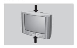
The VOLUME - + (-  $\checkmark$  +) keys are used to adjust sound levels. The PROGRAM - + (-  $\checkmark$  + or - +) keys are used to select the required programmes. To access the menus, simultaneously hold down the  $\checkmark$  - and  $\checkmark$  + keys. The PROGRAM - + keys may then be used to select an adjustment and the -  $\checkmark$  + keys to make that adjustment. To exit from the menus, hold down the 2  $\checkmark$  -
