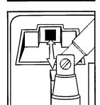
• Fix the indoor aerial at the mounting-socket located at the top left of the rear panel of the TV (unless an outdoor aerial is to be used).
