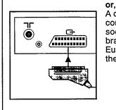
A device with a Euroconnector can be connected to the Euroconnector socket at the back of the TV (a support bracket is provided for the Euroconnector cable on the back of the TV).
