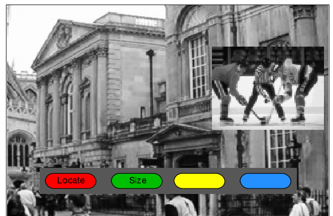
The PIP picture has been moved to an alternative position and made smaller by pressing the Locate key twice followed by the Size key once.
