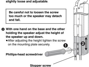
Screw to stop mounting plate from moving or sliding below this point.
