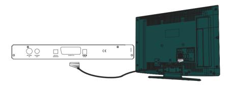
Connect your set-top box with a scart cable using the TV scart connector on the rear panel to your television's scart connector. The set-top box gives RGB or CVBS output. If you want to get the picture via scart connector and your TV's scart connector has an RGB input, then you can switch your digital set-top box to RGB mode, by toggling TV out menu to RGB mode, in configuration menu. So, you will be able to achieve high performance from your digital set-top box.
