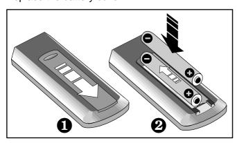
**Note:** Remove the batteries from the remote control handset when it is not going to be used for a long time. Otherwise it could be damaged if the batteries leak.
