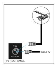
Connect the aerial or cable TV plug to the Aerial socket located at the back of the TV. If you are also connecting a VCR, plug the aerial cable into the aerial input socket on the VCR and then connect the RF output cable from the RF out socket on the VCR to the TV aerial socket. See Page 20 for further details.
