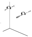
NOTE: You will need to ensure the screws are long enough to sufficiently grip the wall while allowing 5mm between screw head & wall.
